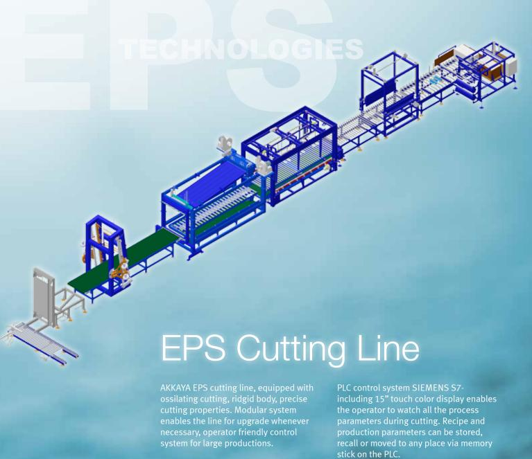
Special designed hot wire ossilation, has a automatic speed control system during cutting. This gives the change for fast cutting without any wire break. This option installed only on horizontal cutting station.
